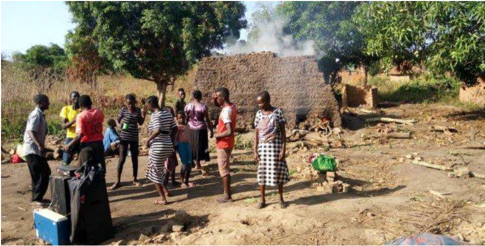
Photo 3: A youth group in Yambio is burning clay bricks for construction (credit: Matthias Fettback)
